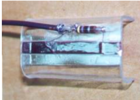
Figure ♦ . ♦ The finished loop with tape added to protect the magnet wire
